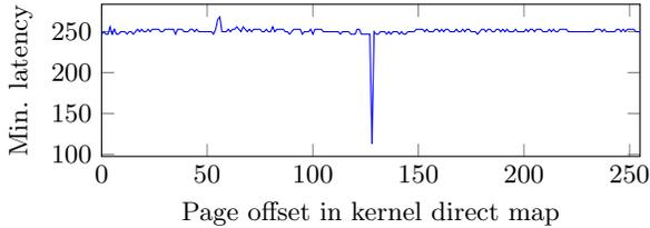
**Figure 3: Minimum memory access time for an address  $p$  after prefetching different inaccessible addresses, on an i5-3320M. Peak shows the single address  $\bar{p}$  mapping to the same physical address as  $p$ .**
