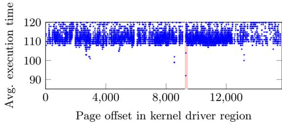
**Figure 9: Second stage: driver region is searched by measuring average execution times of prefetching addresses in the driver memory area from the first stage. Lowest average execution time is measured on an address in the memory of the targeted driver.**
