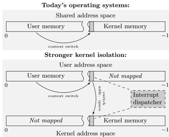
**Figure 10: Currently kernel and user memory are only separated through privilege levels. With stronger kernel isolation, the kernel switches from the user space to a dedicated kernel space, directly after a context switch into privileged mode. Thus, only a negligible portion of interrupt dispatcher code is mapped in both address spaces.**
