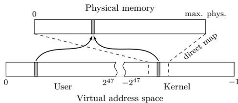
**Figure 1: Direct mapping of physical memory.** A physical address is mapped multiple times, once accessible for user space and once in the kernel space.
